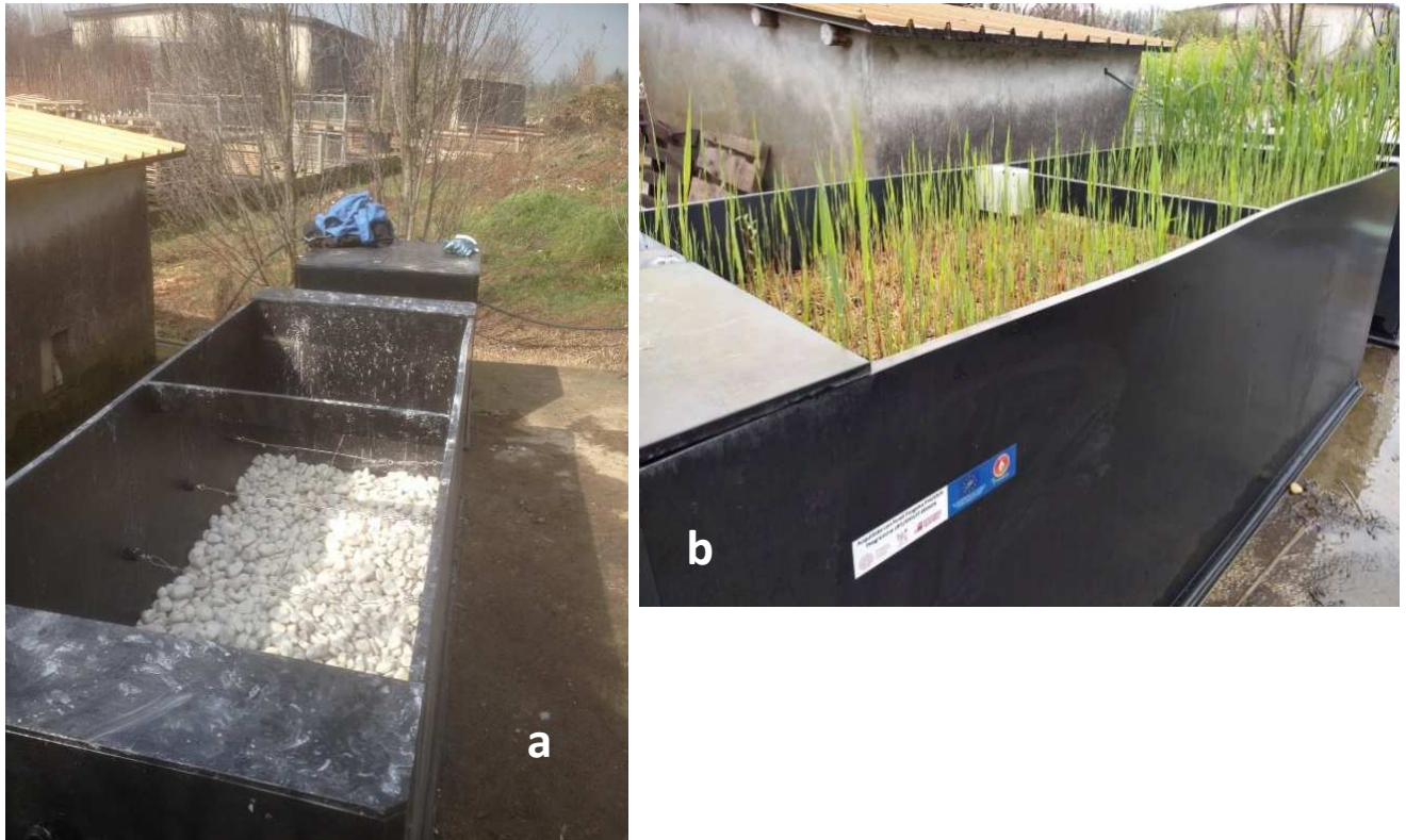
Figure 30. Phytoremediation pilot plant Main tank: a) during the preparation with layers of stone; b) with young plants of Phragmites australis planted for a few weeks
