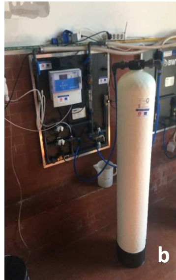
Figure 27. Pilot plant: a) control panel; b) regenerable ion exchange resins
