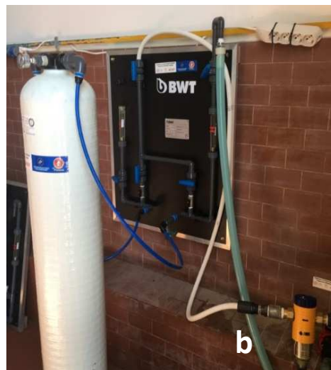
Figure 28. Pilot plant: a) control panel; b) non-regenerable ion exchange resins
