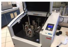
LIFE PHOENIX: a planetary mill for soil analysis in ARPAV laboratories. An innovative tool that allows the simultaneous preparation of multiple samples.
